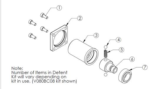
"Item 5" is the detent spring that must be replaced with the new "soft" spring, P/N 0602025333M1.
